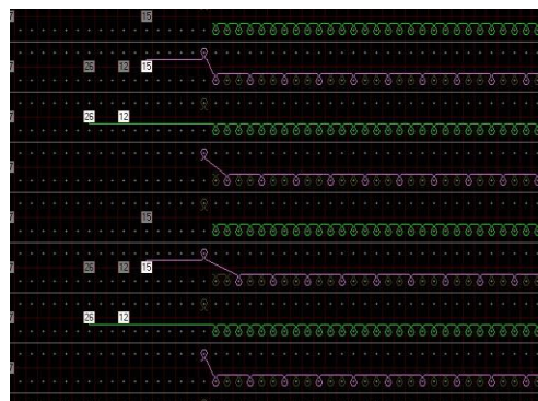
Fig.10. Representation by row section – yarn carriers
