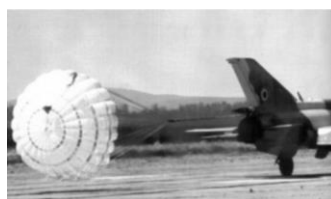
Fig. 2: Parachutes for landing and deceleration of the supersonic aircraft
