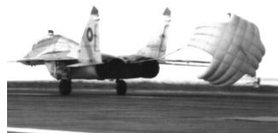
Fig. 2: Parachutes for landing and deceleration of the supersonic aircraft
