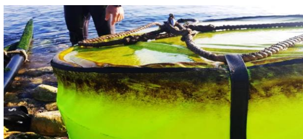
Fig. 6. Deposition of epibiosis on ME1 - floating element located offshore
